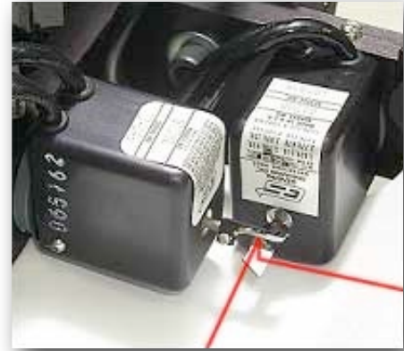
A projector uses two galvanometer scanners, one for horizontal (X-axis) and one for vertical (Y-axis). The photo shows two General Scanning model G-120 scanners. The laser beam enters from the right, is deflected first by the X-axis mirror and then by the Y-axis mirror, and finally exits towards the viewer or projection screen. Photo courtesy Pangolin Laser Systems Inc.
